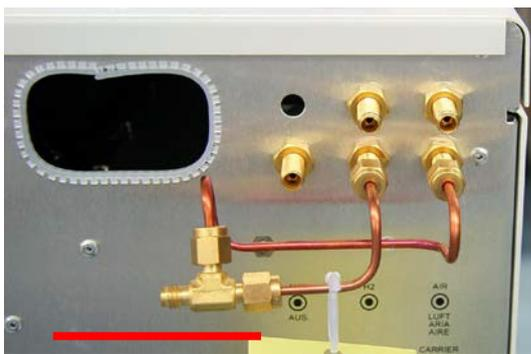
**Air tubing from the solenoid is connected to the AIR (left)**
