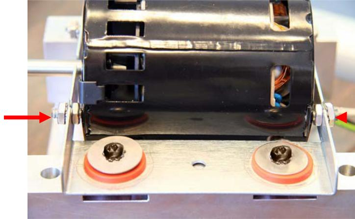
6. Tighten (with a wrench) all 4 **INNER NUTS** into direction of the motor mount.
