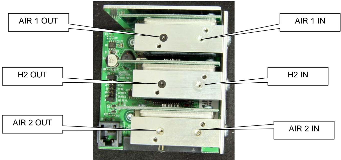
This section contains illustrated parts breakdowns for the 436-GC/456-GC Gas Chromatograph Manual flow control and related components
