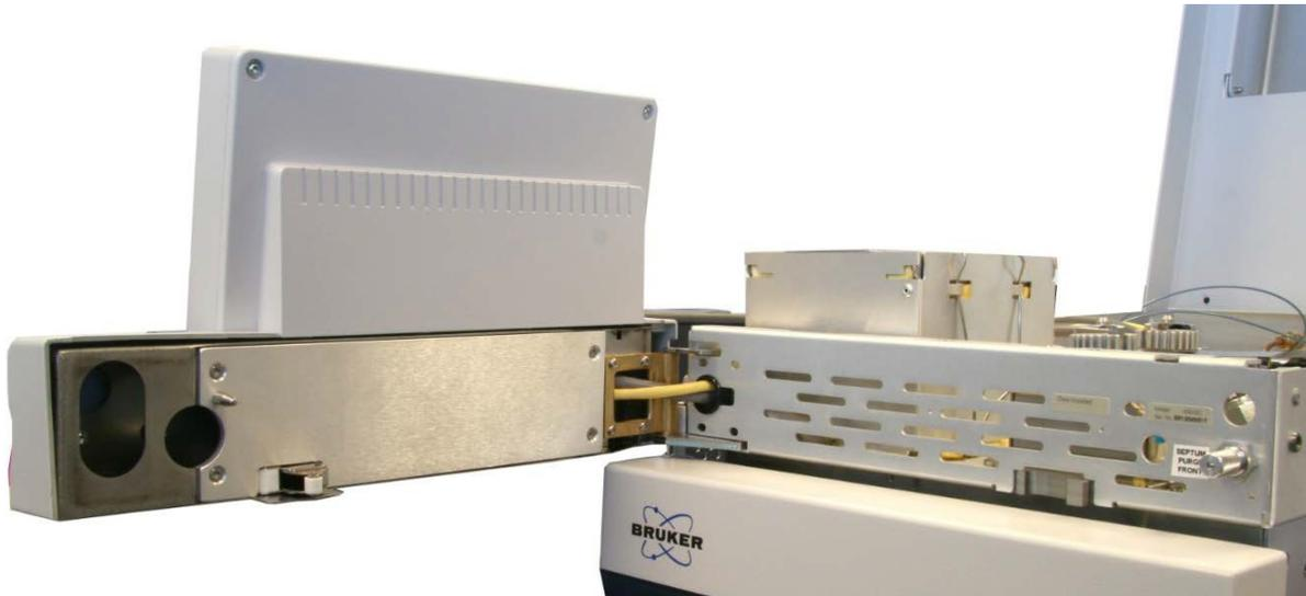
2. Loosen the 4 Torx screws from the lid covering the LUI compartment.
