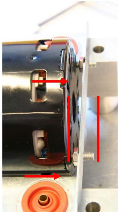
4. Check and correct if necessary (with the inner nuts) if the fan motor housing is parallel with the motor mount.
