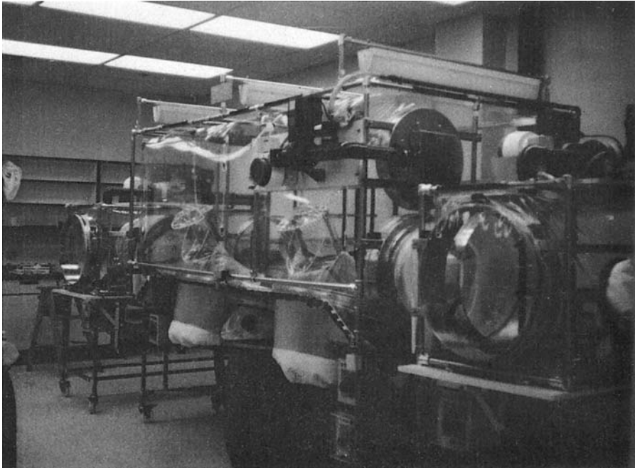
Fig. 1.8 Example of a LaCalhene isolation barrier system for sterility testing (courtesy of Eli Lilly and Co., Indianapolis, Indiana).
