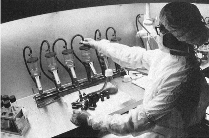
Fig. 1.5 Set-up of the classic membrane filtration sterility test apparatus. (Courtesy of Eli Lilly Co., Indianapolis, Indiana.)
