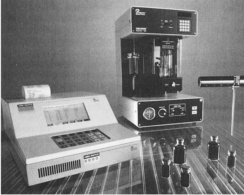
Fig. 3.9 HIAC/Royco's System 8003 for parenteral particle counting to comply with the requirements of microscopic particles. (Courtesy HIAC/Royco Division of Pacific Scientific Company, Silver Springs, Maryland.)
