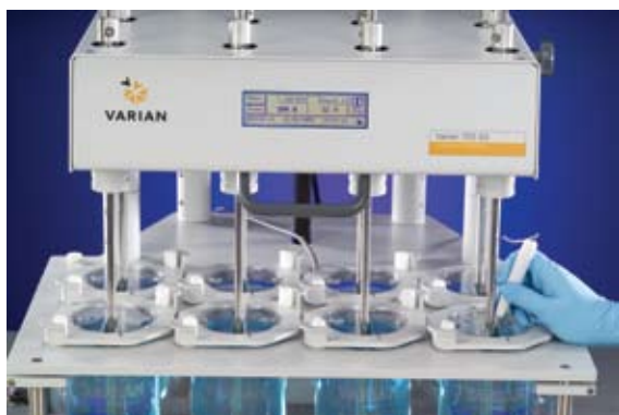
Individual Vessel Temperature Measurement
