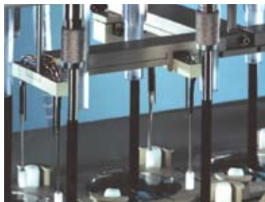
Motorized Sampling Manifold
