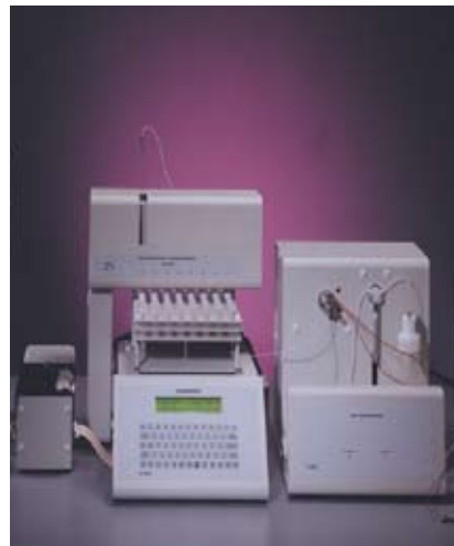
Pump, VK 8020 Sample Collector, and Auto-Injection Station
