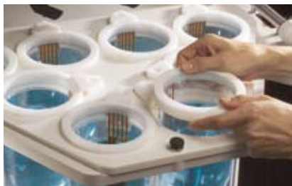
Direct Vessel Heating Vessels (DVH)
