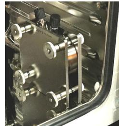
By using the migration cell System-Siegwerk (Sieg-Mi-Flex), a migration estimate of the packaging contents from food packaging can already be conducted using the finished rolls of material.
