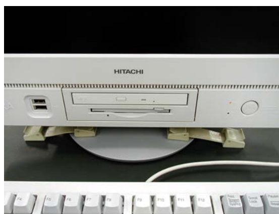
Fig. 1-3. Example of securing personal computer
